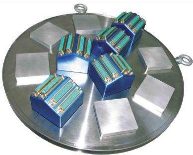
ISO K DN500 Flange equipped with 11 x 4x50D-SUB wired feedthroughs 2200 signals
