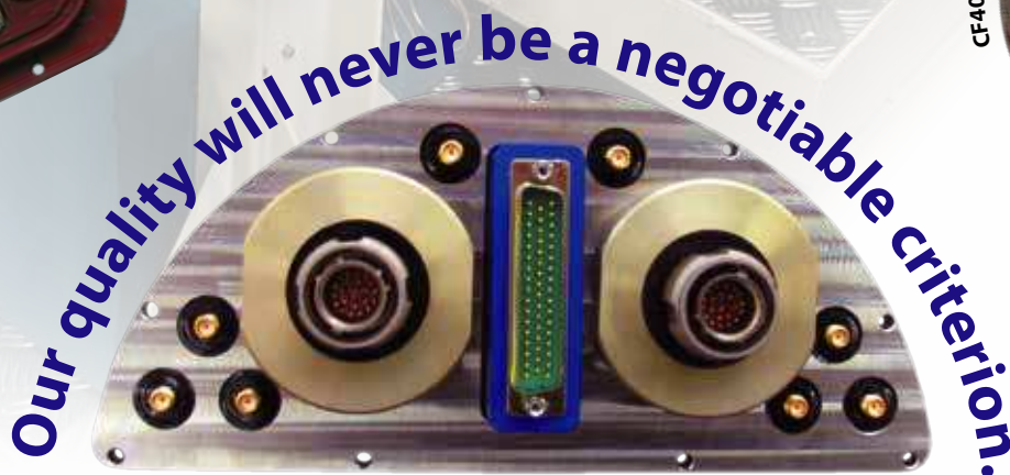
Custom design flange - 2 x MoR M45 D38999 - 1 D-SUB 50 ND Ev and 8 x SMA 18 GHz
