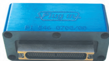
Custom designed 120 pins ERVAC module
